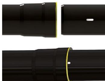
It is easy to cut the pipe to the desired lengths. Connectors can be used to connect sleeveless pipes that have been cut. This minimises the loss of pipe. Due to the innovative structure, a sleeve joint used in Allaway dust piping is also achieved when using a connector.
